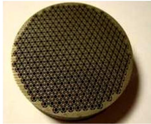
Fig. 13: Compact heat exchanger realized through SLM process
